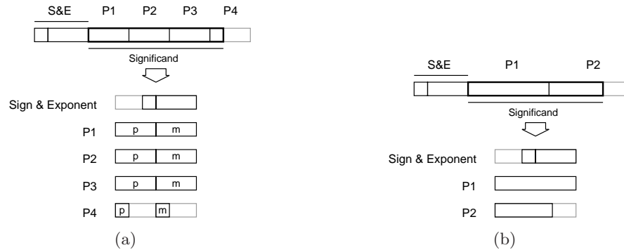
Figure 6. (a) Quantization of double precision type into packets for a 32-bit wide machine implementing OFPA. Note that packet P4 is partially filled as there are more digits available to four packets than present in a double precision type (b) Quantization of double precision type into packets for CFPA.
